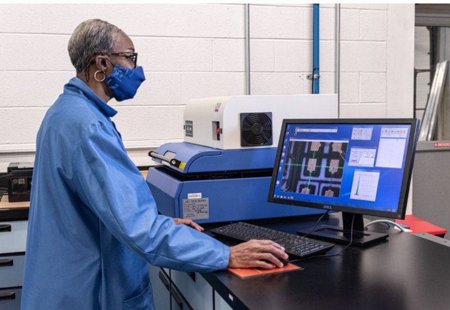
XRF X-ray fluorescence—Micro Pioneer XRF 2000.
