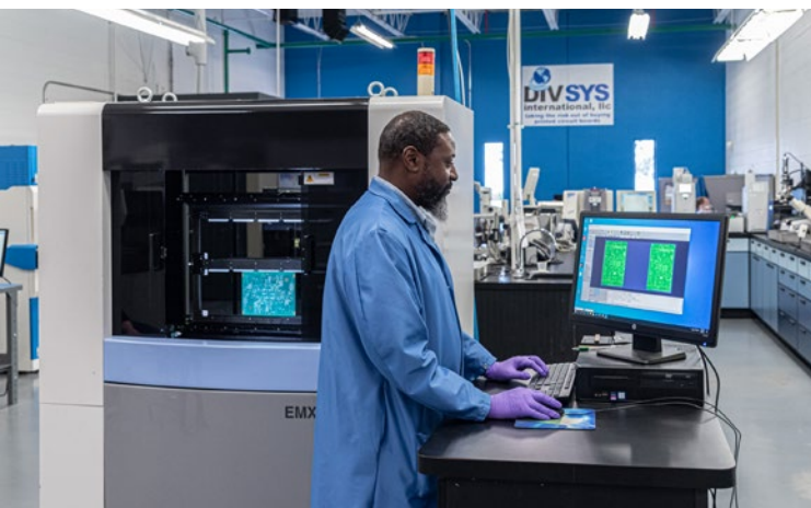
Bare board electrical test— MicroCraft EMX6151 Flying Probe.
