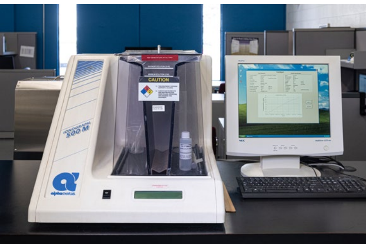
Ionic contamination— SCS Alpha Metals 500M Ionograph.
